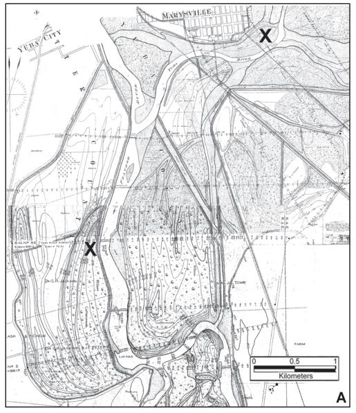
Figure 12. Channelization around Yuba-Feather confluence. Several ditches were dredged south of Marysville shortly before 1909. Two ditches connected with the Feather River at Elisa Bend, and another turned the confluence south. (A) Stratigraphic sections collected at Xs are shown in Figures 13 and 15A. (Source: CDC, 1912.) (B) Ditches are prominent (cartographically exaggerated) on 1914 map. (Source: Crook, 1914.)
