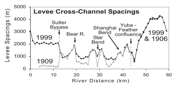
Figure 3. Levee cross-channel spacings in 1999 in comparison with 1909 (Feather River) and 1906 (Yuba River). Measured from 1999 DOQQs and California Debris Commission (CDC) 1906 and 1912 maps.
